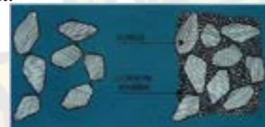
Fig 4: Pores occupied by Silica Fume
